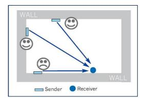
**Tip 5** Avoid radio propagation along a wall (also given in a long narrow floor).
