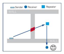
Avoid an unfavourable penetration angle by repositioning the transmitting and/or receiving antenna, or by using a repeater.
