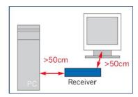
Tip 7 The distance of the EnOcean receiver to different high-frequency transmitters should be at least 50 cm, the transmitter position is not critical. No 868 MHz power RFID and 868 MHz EnOcean receivers in the same room.
