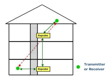
In rare cases of heavily reinforced concrete ceilings or thick basement walls a second repeater may be necessary to ensure full coverage (both repeaters must be switched to 2-level function, see information in chapter 1.6).
